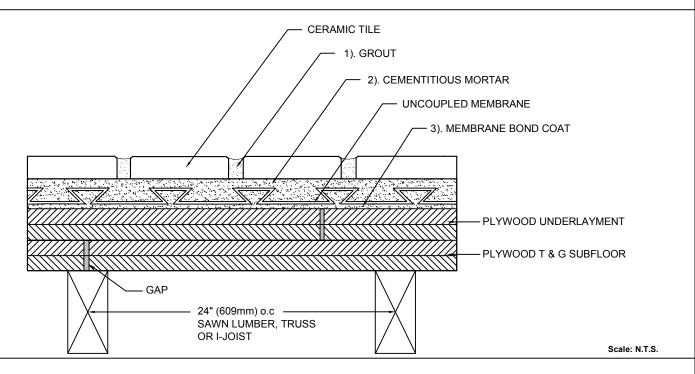
Drawings are developed to be compatible with Tile Council of North America 2013 TCNA Handbook for Ceramic, Glass and Stone Tile Installation.
