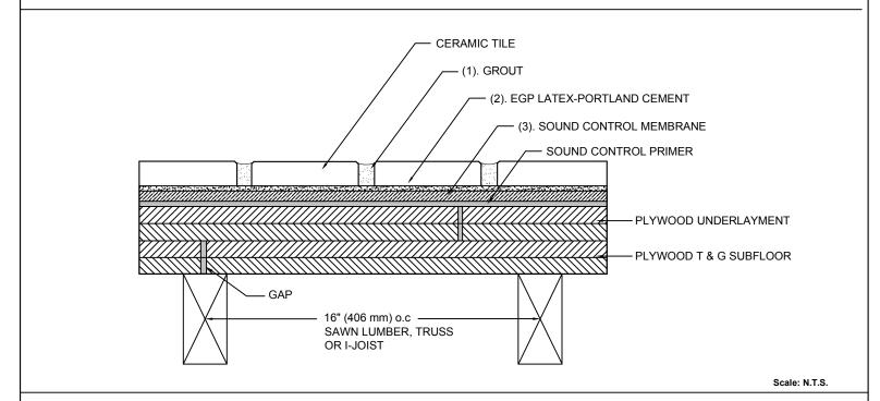
Drawings are developed to be compatible with Tile Council of North America 2013 TCNA Handbook for Ceramic, Glass and Stone Tile Installation.
