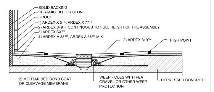
SHOWER RECEPTORS, CURBS, SEATS, ETC. MUST BE PROPERLY WATERPROOFED AND INSTALLED TO AVOID WATER DAMAGE TO ADJACENT BUILDING MATERIAL. SEE TCNA COMMON SHOWER CONFIGURATIONS SECTION.
